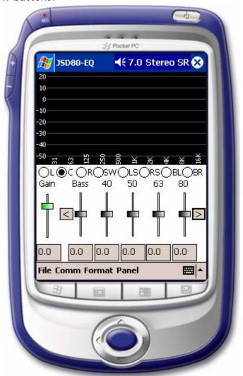
To make an equalizer adjustment select the appropriate channel and scroll left or right to the appropriate band and slide the level up or down.
