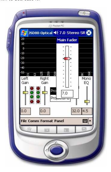
The Inputs form has been broken down into two independent forms, one for adjusting optical preamps and the other for matrix adjustments. The following screen illustrates the Optical preamp adjustment form.
