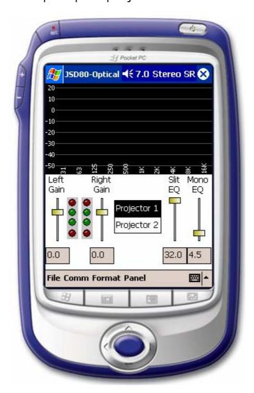
The left and right gain adjustment controls are used to adjust the preamp input levels for optical film modes. The led indicators are used in conjunction with A-chain alignment for setting the proper level with a 1k test tone input. The Projector 1 and Projector 2 buttons allow you to select which projector preamp you want to adjust. Slit EQ and Mono EQ adjustments can also be made to the preamp adjustment.
