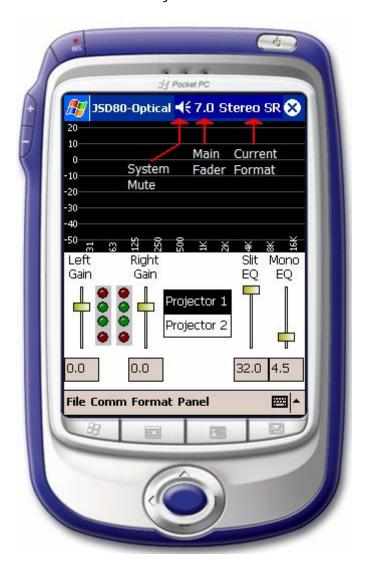
The following illustration shows the main fader adjustment when the mainfader control is tapped. Move the slider control up to increase main fader volume and down to decrease it.
