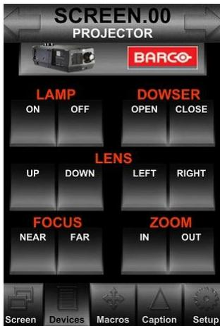
The PROJECTOR touchscreen contains common projectionist controls to remotely adjust the projector's lamp, dowsers, lens movement, focus, and zoom settings.
