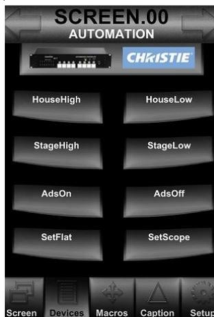
AUTOMATION devices are configured with predefined command scripts that are used to control various types of theatre equipment in an auditorium. A defined automation command type is activated by touching the respective button in the AUTOMATION touchscreen. As shown, the user can control items such as the house lights in an auditorium.
