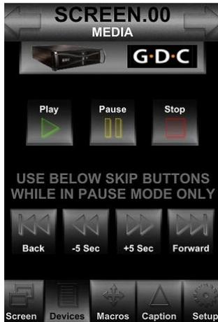
From the MEDIA touchscreen you can control the media server. This allows the content playing to be paused / un-paused as well as being able to skip forward and backwards in increments of five seconds.
