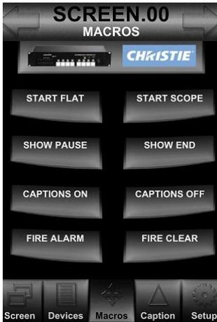
Automation devices are configured with predefined command scripts that are used to control various types of operations in an auditorium. A script is executed by sending a defined command cue (a macro) which is stored in the RTP-100 Wireless Server Module and activated by touching a button from the MACROS or other touchscreens.
