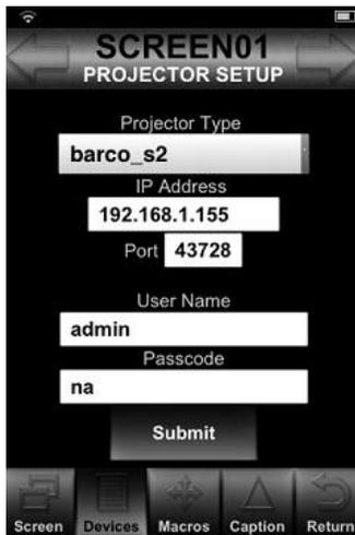
After entering the configuration settings, activate the **SUBMIT** button and wait for the RTM-100 to update. When this action is complete, the **MAIN MANAGER** screen will display.
