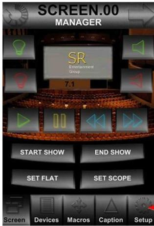
The SETUP button is used to open the configuration setup screen for the selected items available for screens, devices, macros, and captions. When the SCREEN MANAGER is selected and the SETUP is activated, the configuration settings screen is displayed. For each screen number / auditorium, a configuration may be set. There is ability to enter a name for a given auditorium via the configuration screen.
