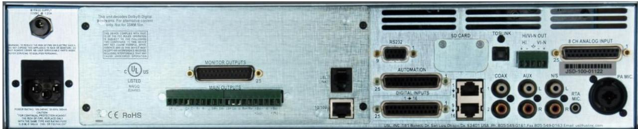
JSD-100x with 8 analog channel output module
