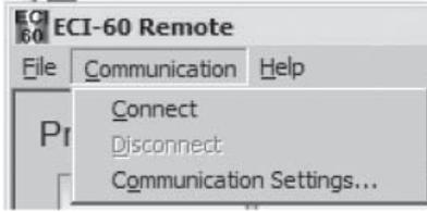
In the “Communications” tab you may choose to “Connect” to an ECI-60 or configure your “Communications Settings” When changing communications settings, the ECI-60 must not be connected to the setup software.
