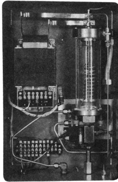
**BOILER ASSEMBLY, TRANSFORMER, Etc.**
