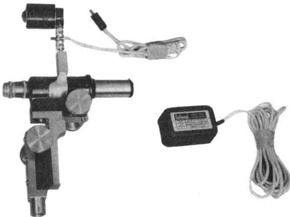
This Comparator Telescope is used primarily on baths when testing etched stem thermometers. The Comparator Telescope can be moved from bath to bath providing each bath is equipped with a telescope stand.
