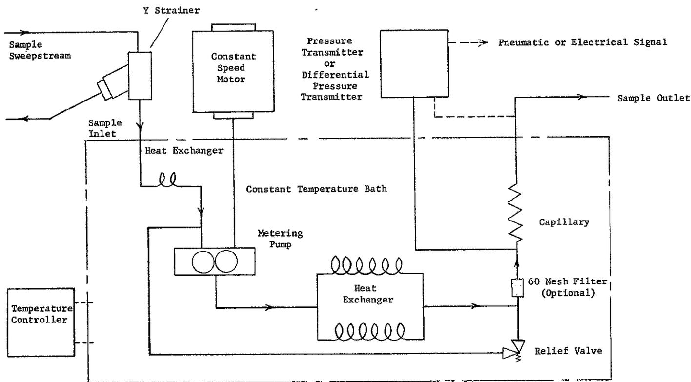
**Figure 1 — Schematic Flow Diagram**
