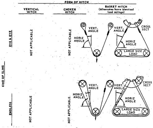
NOTES: For vertical angles of 5° or less, refer to Figure N-184-4 "Basic Sling Configurations with Vertical Legs".
