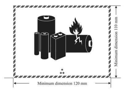
(A) The mark must be in the form of a rectangle with hatched edging. The mark must be not less than 120 mm (4.7 inches) wide by 110 mm (4.3 inches) high and the minimum width of the hatching must be 5 mm (0.2 inches) except markings of 105 mm (4.1 inches) wide by 74 mm (2.9 inches) high may be used on a package containing lithium batteries when the package is too small for the larger mark;
