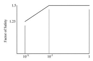
P<sub>i</sub>, Probability of occurrence of failure mode j (per hour)
