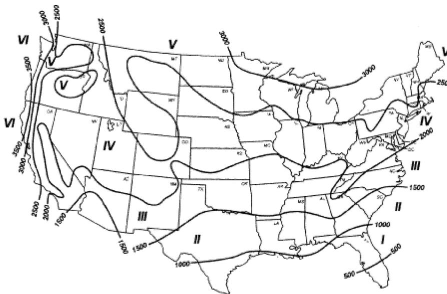
Figure 1—Heating Load Hours (HLH<sub>A</sub>) for the United States
