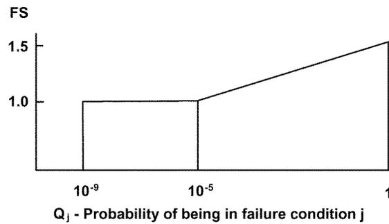
Figure 2: Factor of safety for continuation of flight
