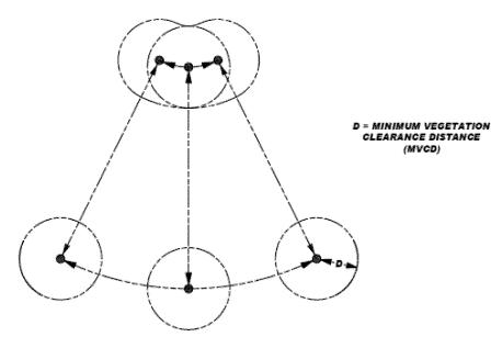
NERC indicates that conductor movements must be taken into account under FAC–003–2, and that the transmission owner is required to show that its approach to vegetation management under Requirement R3 will prevent encroachments under all expected line positions. <sup>105</sup> Thus, a transmission owner must manage vegetation to ensure it does not encroach into the MVCD under multiple conditions.
