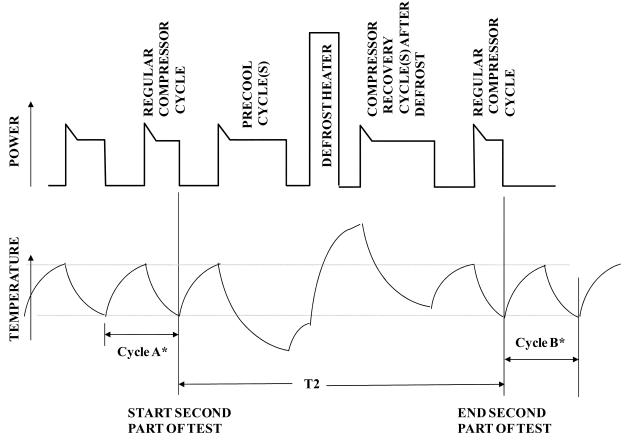
\*Average compartment temperature(s) during cycles A & B must be within 0.5 °F of the average temperature(s) for the first part of the test.
