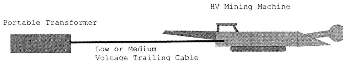
Figure 1-Power Source-75.829(c) (1) 995 volts used for trammimg
