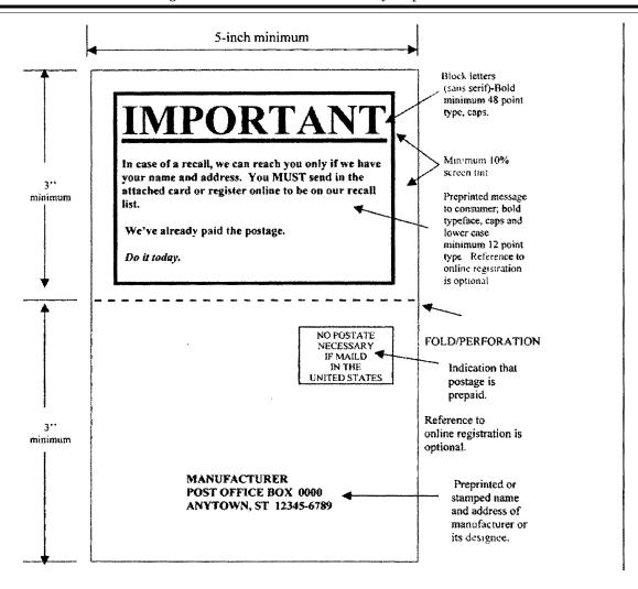
Figure 2 – Registration form for child restraints systems – address side
