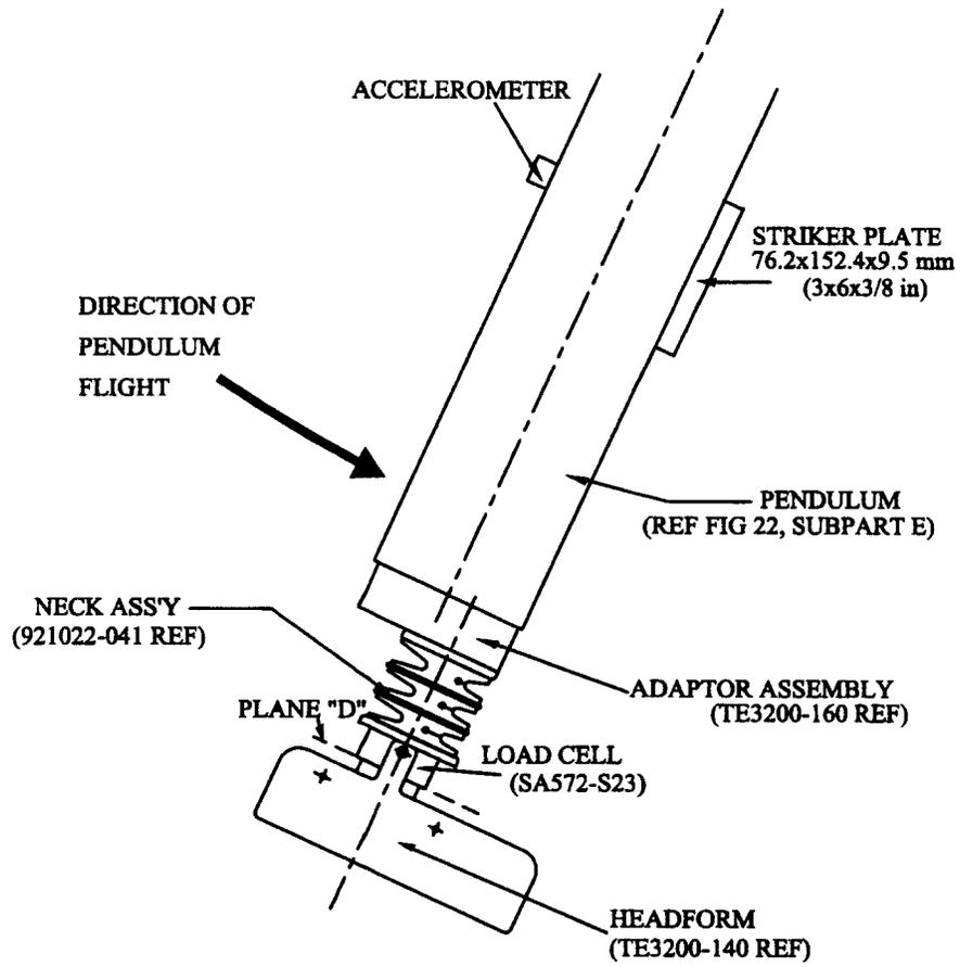
**NOTE: MOUNT NECK AT LEADING EDGE OF PENDULUM TO AVOID INTERFERENCE.**
