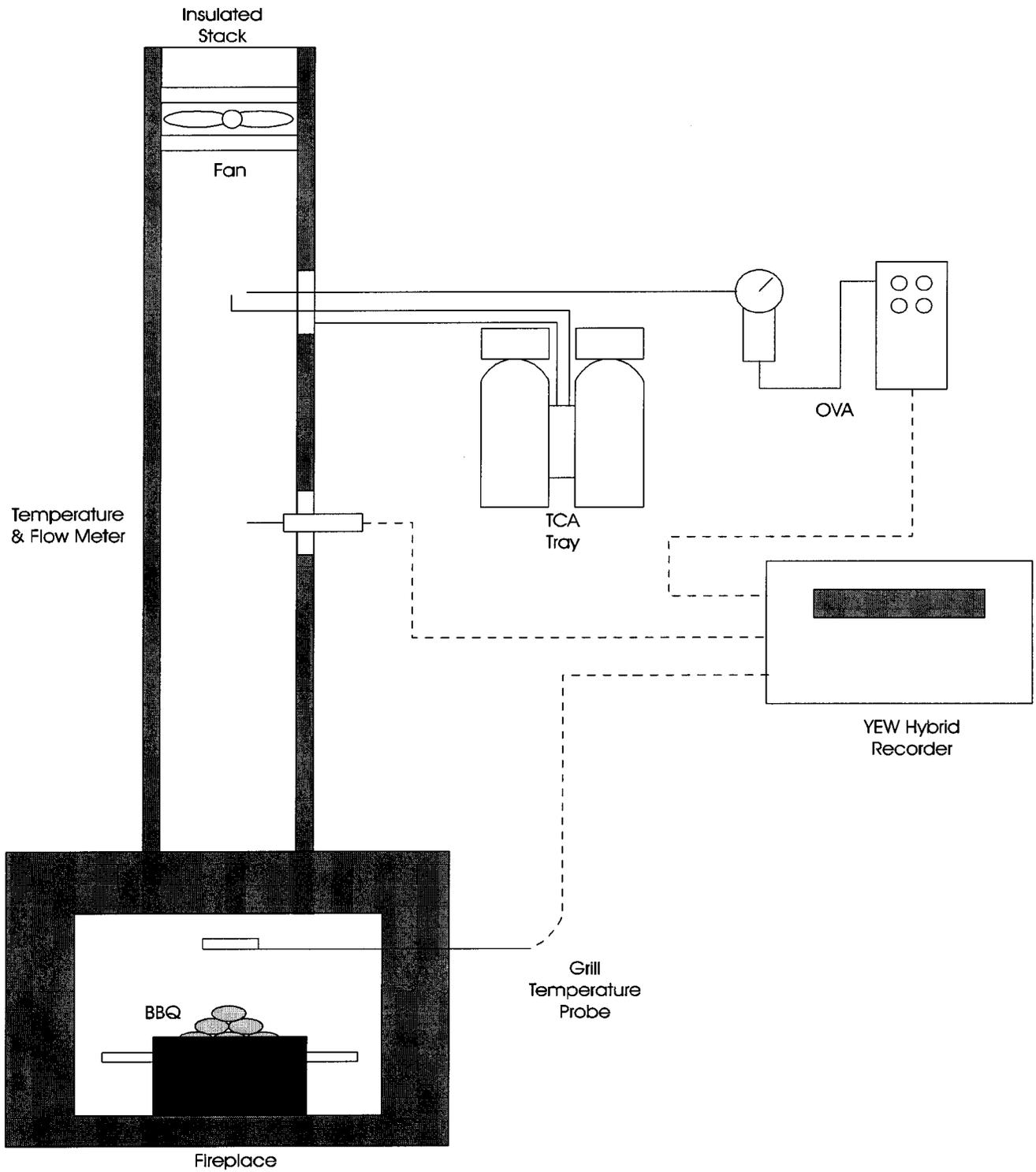
Figure 3. Sampling Apparatus Set-up with Chart Recorder
