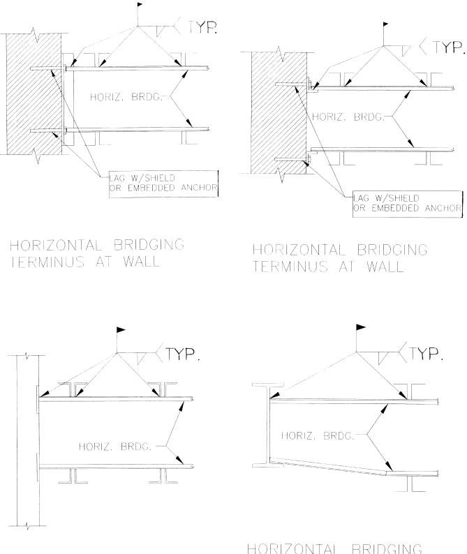
HORIZONTAL BRIDGING TERMINUS AT PANEL WALL HORIZONTAL BRIDGING TERMINUS AT STRUCTURAL SHAPE
