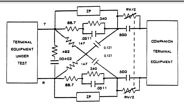
Resistances (Ohms), Capacitances (uF), Tolerances ± 2%.
