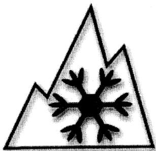
If the manufacturers choose to mark their snow tires with the Alpine Symbol, the mountain profile must have a minimum base of 15 mm and a minimum height of 15 mm, and must contain three peaks with the middle peak being the tallest. Inside the mountain profile, there must be a six-sided snowflake having a minimum height of one-half the tallest peak.
