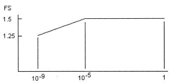
Pi - Probability of occurrence of failure mode i (per hour)
