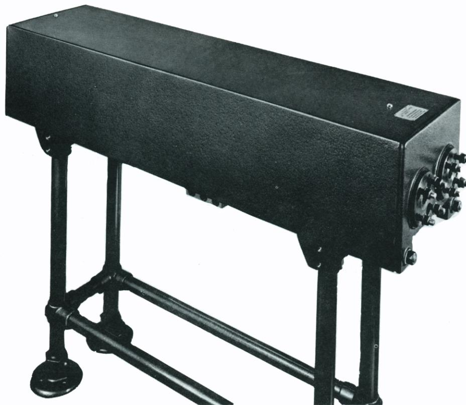
This instrument has been successfully applied to a great many industrial density measurement problems. It provides the most practical method of measuring the density of a slurry and is, of course equally suitable for use with clear liquids.
