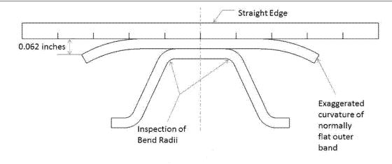
Figure 1 to paragraphs (h)(1)(iii) and (v) of this AD: Cross section of v-band
