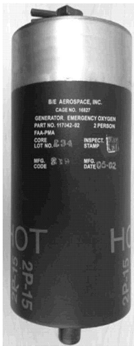
Figure 2 to paragraph (g) of this AD – Manufacturing (MFG.) date (05-02 = May 2002) example
