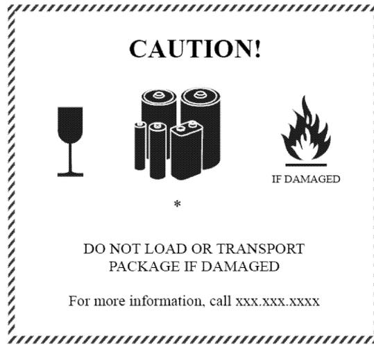
(A) The marking must be not less than 120 mm (4.7 inches) wide by 110 mm (4.3 inches) high except markings of 105 mm (4.1 inches) wide by 74 mm (2.9 inches) high may be used on a package containing lithium batteries when the package is too small for the larger mark;
