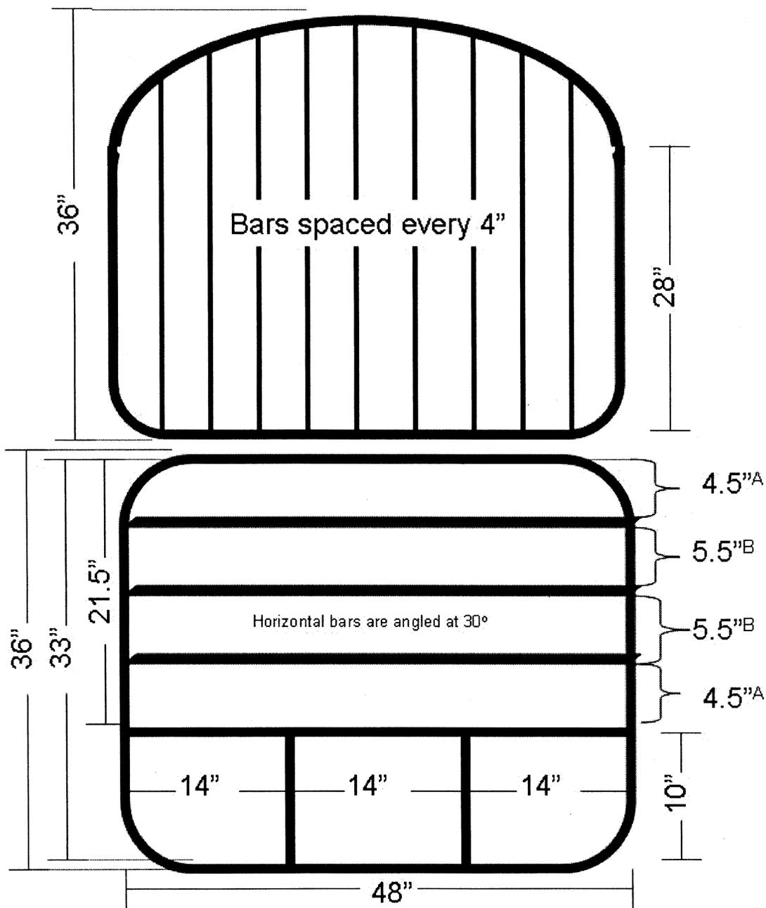
All pipe must be a minimum of 1.25" O.D.; horizontal flat bars shall be a minimum of 1.5" x 0.375"; vertical flat bars shall be a minimum of 1.25" x 0.375"
