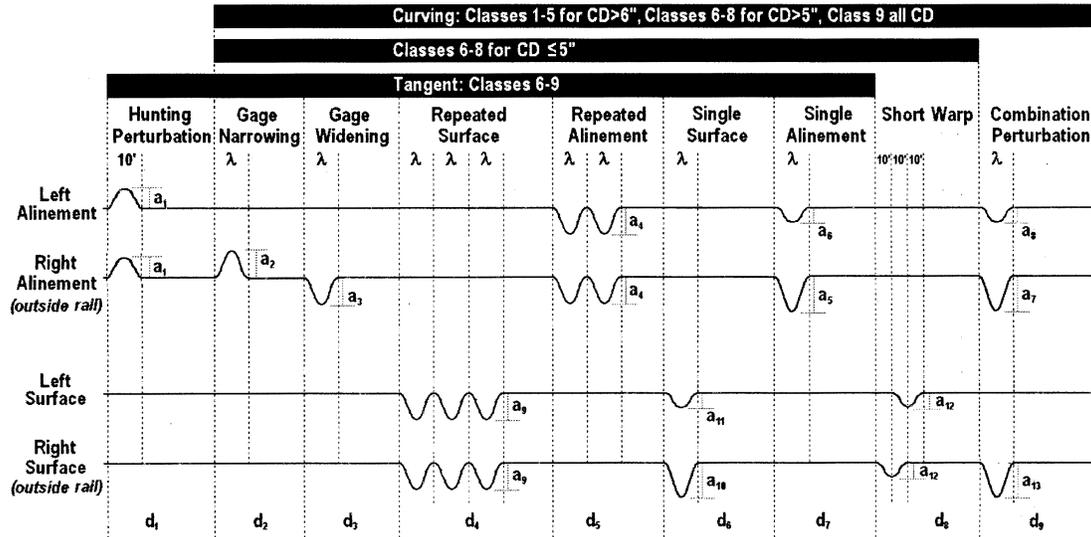
(1) *MCAT segments.* MCAT's nine segments contain different types of track deviations in which the shape of each deviation is a versine having wavelength and amplitude varied for each simulation speed as further specified. The nine MCAT segments are defined as follows:
