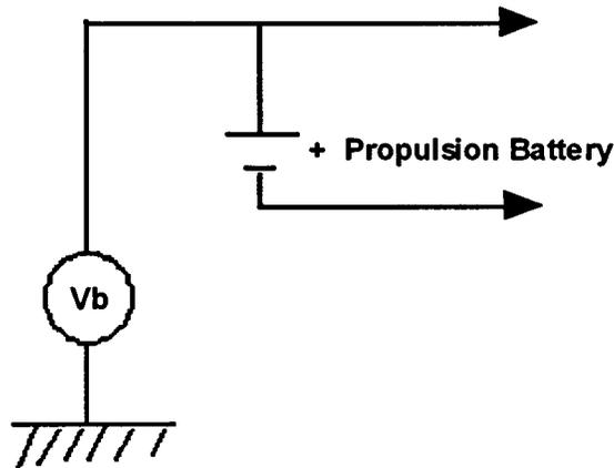
**Fig. 3 S7.7.5 MEASUREMENT LOCATION FOR V2 VOLTAGE**
