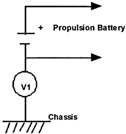
**Fig. 2 S7.7.4 MEASUREMENT LOCATION FOR V1 VOLTAGE**
