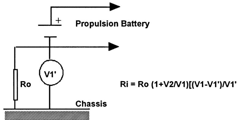
**Fig. 4 S7.7.6 MEASUREMENT LOCATION FOR V1' VOLTAGE**
