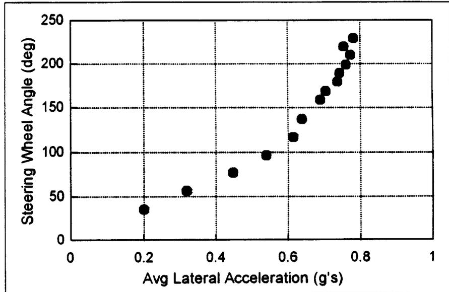
Figure 8. Steering Wheel Angle vs. Lateral Acceleration, 40 mph, 1996 Acura SLX w/o Outriggers.
