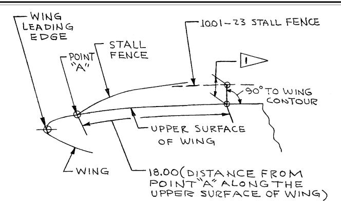
IE STALL FENCE IS 1.16 ± .12 HIGH THAT IS CORRECT HEIGHT FOR CESSNA 150/152. IF GREATER THAN 1.28 HIGH REMOVE STALL FENCES AND INSTALL THE CORRECT ONE.
